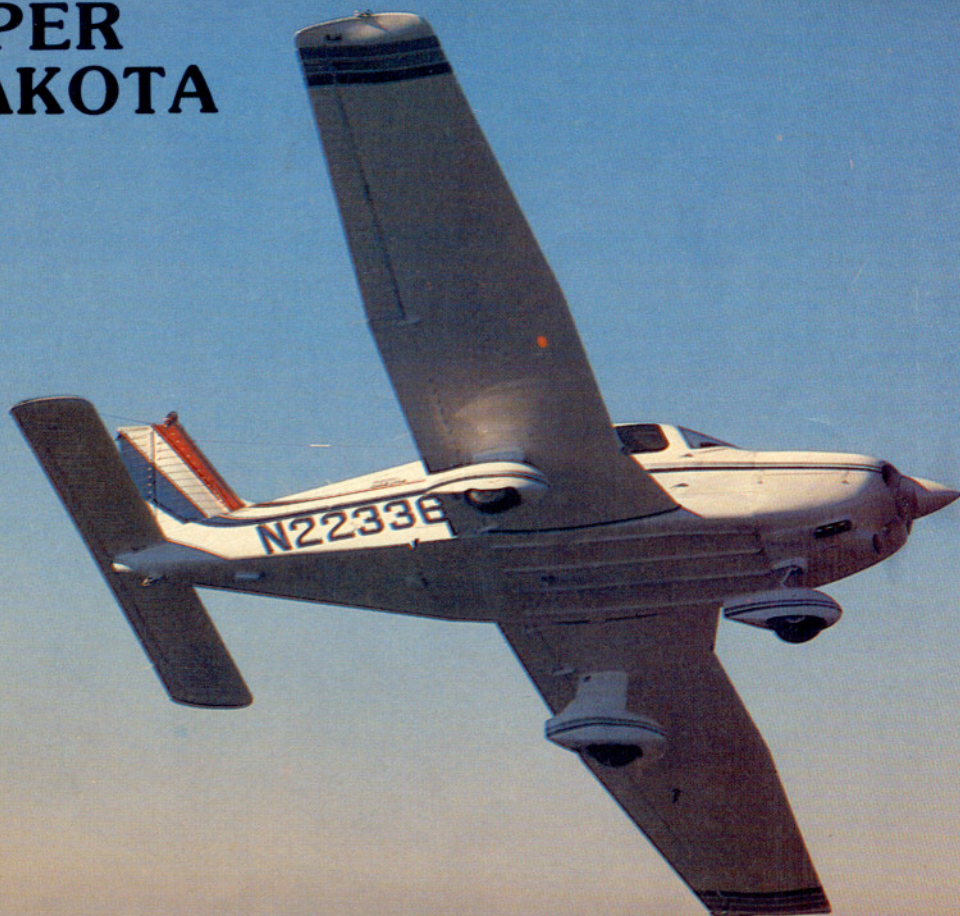
The Dakota shares the longer span, semitapered wing with the Archer, Arrow, Seminole and Warrior. The longer ailerons provide more effective roll control than the original wing used on the Cherokee line.
