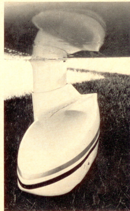
The new, aerodynamically efficient wheel fairings improve cruise speeds by 8 knots and range by 6% over a bare-wheeled Dakota, but they extract a price in terms of more care to check tire inflation and condition.
